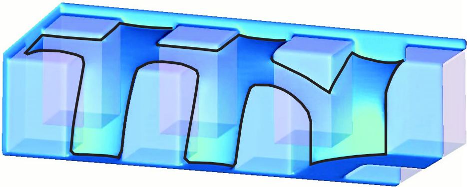
Figure 11. The curvature of the liquid-gas interface is visualized by numerical results performed in 3D. Liquid from the reservoir above pushes away the gas (below the contoured area) from top to bottom and right to left. The front pillars are made transparent. This numerical simulation was performed by Mauro Sbragaglia.
