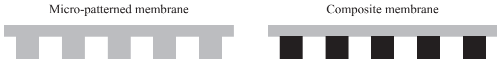
Figure 6. Schematic representation of the cross-section of a micro-patterned membrane (left) and a composite membrane (right) with the same dimensions.
